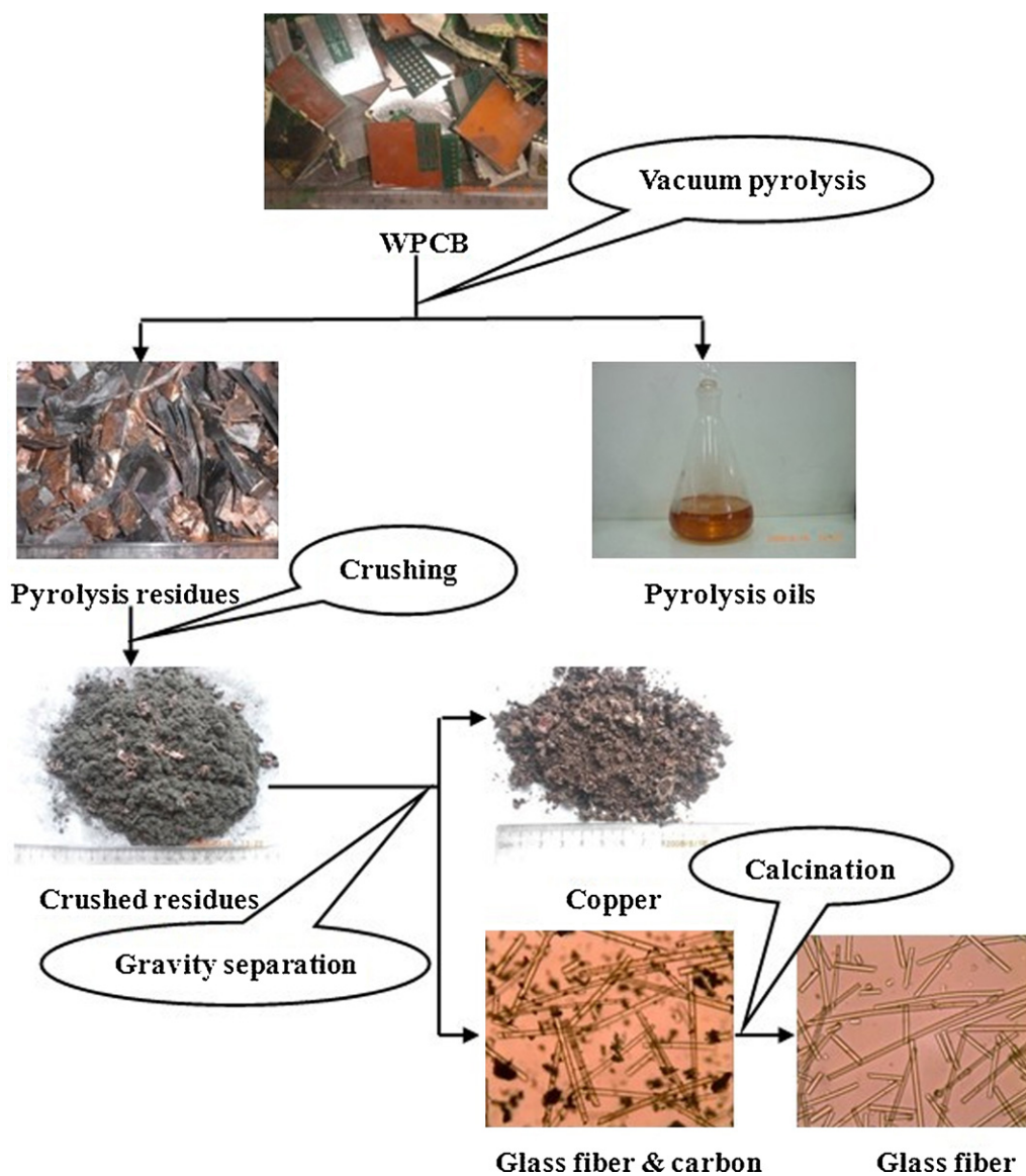
Fig. 4. Schematic illustration of recycling WPCB.
